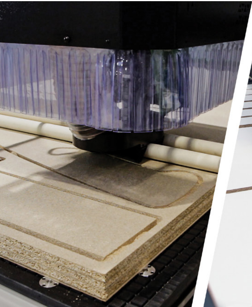
The process of nesting and drilling
